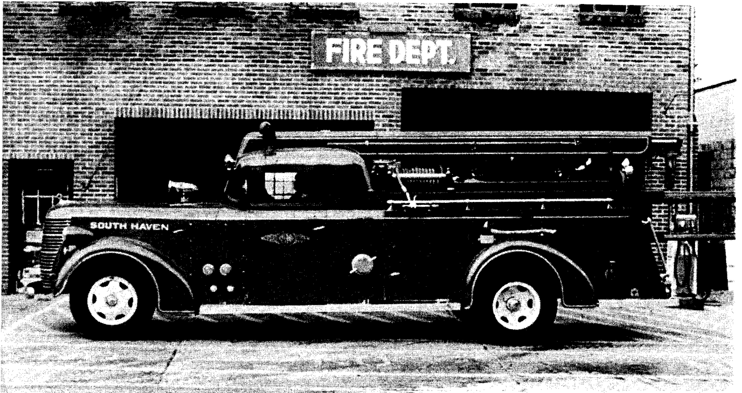
This 1946 model American LaFrance had a 12-cylinder engine capable of pumping 1,000 gallons of water per minute. It remained in service more than a quarter of a century.
