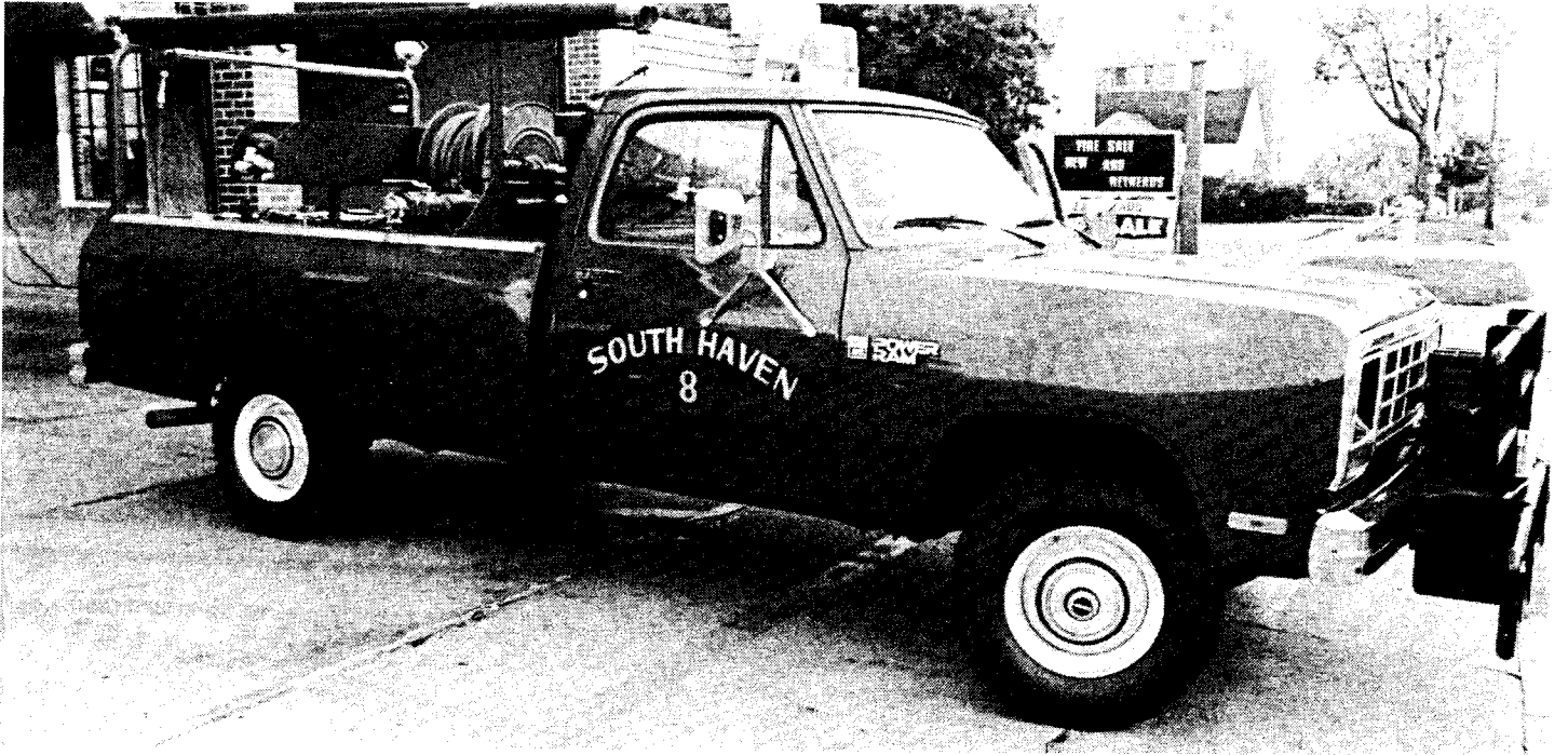
Four-wheel drive grass truck with power winch in front was added to the fleet in 1983.
